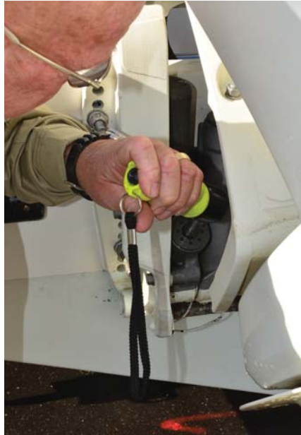
A full inspection includes all outboard systems, not just the engine. Tilt, prop, exhaust, ignition and more should be examined closely.
